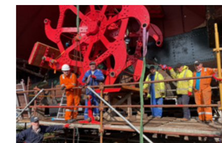
Cover pic: The 1953 paddle steamer Maid of the Loch is hauled out just now on her slipway at Balloch Pier, while she is being restored by a determined and resourceful bunch of volunteers. This team is working on rebuilding the starboard paddle wheel.
